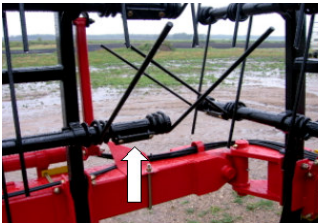
Fig. 6 Harrow Tine Retainers at Boom Joint
