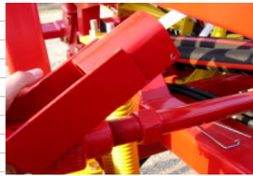
Fig. 3 Screw Jack Lock
