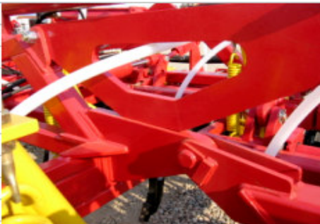
Fig. 8 Over-Center Lock (5710-70 only)
