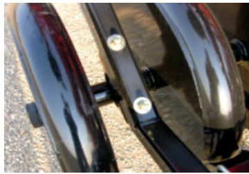
Fig. 2 Pillow Block Bolts (Torque to 75 ft-lbs) (Check 5 randomly)
