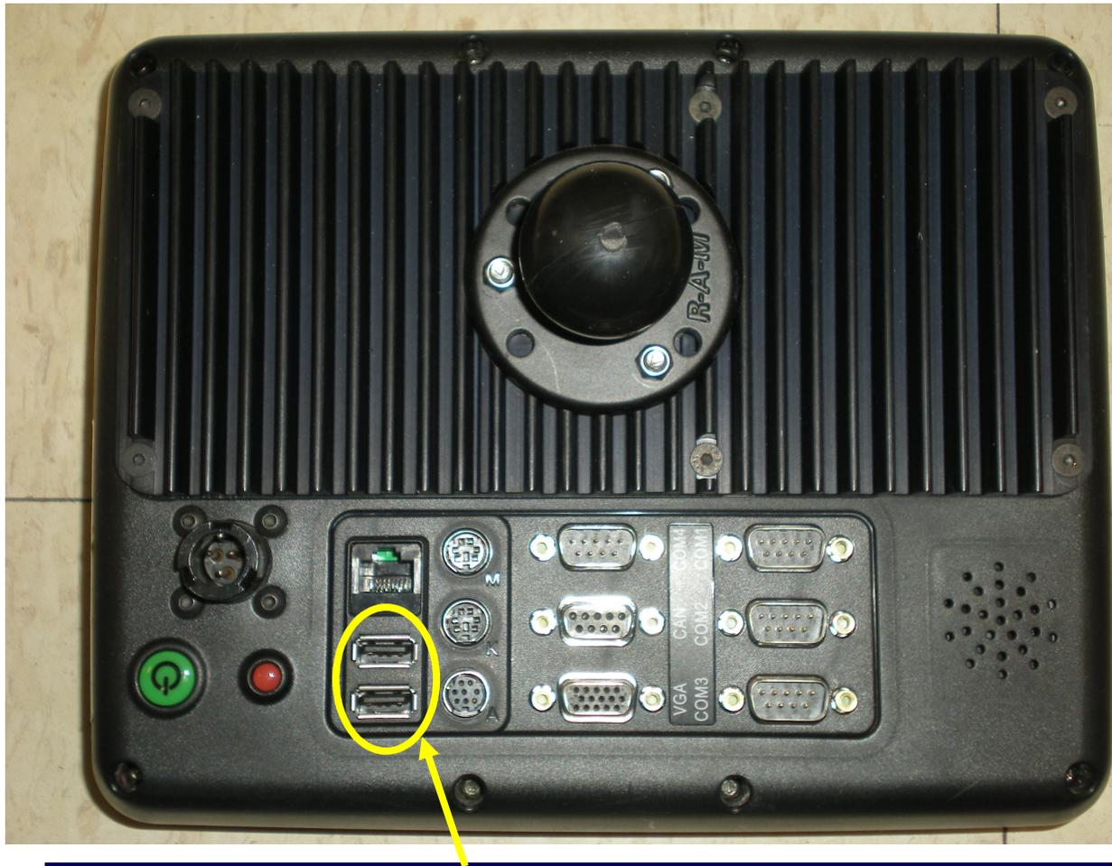
**Step 1 Install a USB memory stick in one of the USB ports.
