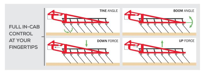
"Since its release in 2017, the Adjustable DownForce System has made the XR harrows the industry leader for performance and ease of setting with in-cab control of all functions." stated Devin Lung, Product Development Leader - Current Products for Bourgault.
