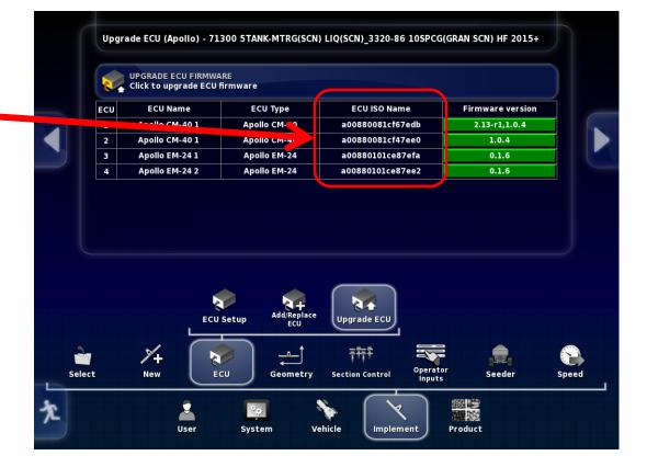
In the right column under Firmware version, select green tab for ECU to be upgraded.
