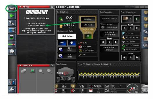
11. On main screen, click the Bourgault button in the top left hand corner. Ensure that the software version shown is correct. (3.24.508)
