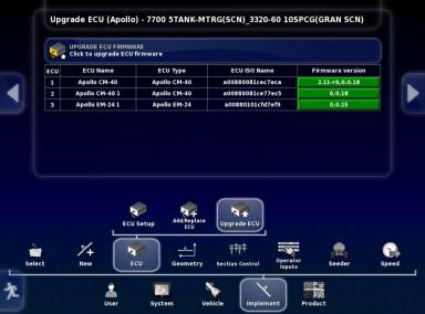
In order to Upgrade the Main Firmware you will have to create an "Upgrade" profile. (Some tanks may already have this profile) Do this after you have Upgraded all ECU's on machine. (Once
