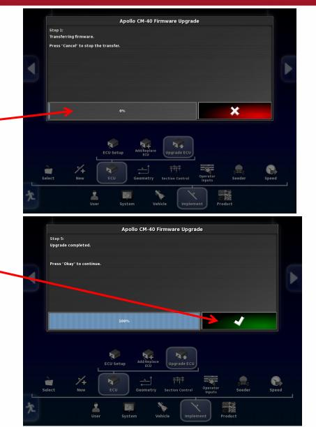
Monitor will restart, Communication will have To be re-established with ECU's ECU's may need power supply removed before they will synchronize. This can be done by shutting tractor off or unplugging ISO plug at rear of tractor
