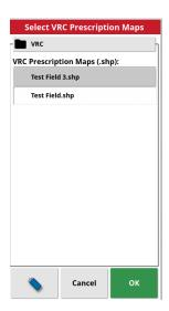
It is now possible to configure the PackMaster control to a VRC prescription. The VRC file is loaded the same way as product applications and can be used either to control pack force or hydraulic pressure. This feature is not recommended to be used at this time unless confidence in gained in the actual desired pack force/hydraulic pressure throughout the field to ensure intended performance.
