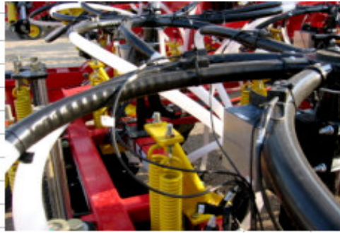
Fig. 10 Blockage Sensor Mounting
