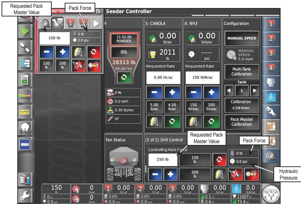
Figure 13.7 - Drill Control - Pack Master Feature
