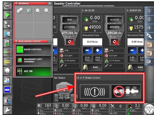
Figure 13.18 - Brake Control Window
