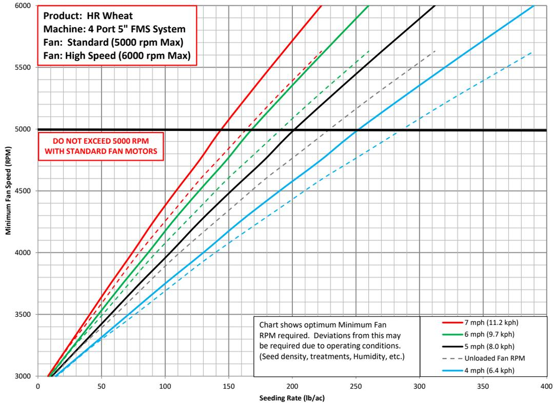
**Note:** FOR RATES BELOW 50 LB/AC USE A MINIMUM FAN SPEED OF 3000 RPM.
