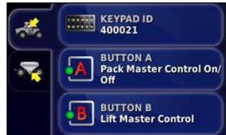
2. Use the provided cabin keypad decal to mark the function of the assigned buttons.
