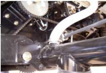
Figure X - Pressurization Line
