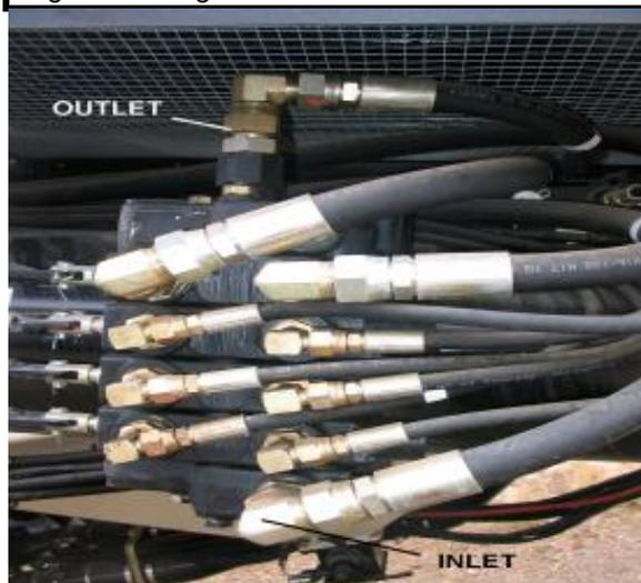
L/U auger manifold hydraulic line layout
