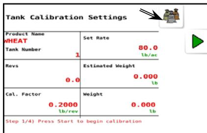
*An initial calibration factor must be entered in order to perform an actual calibration (Refer to calibration factor charts in UT Operator's Manual).*
