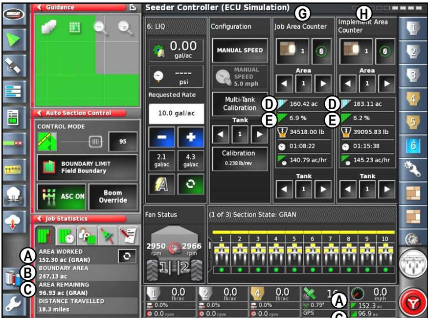
**E - ASC Savings** - Displays the calculated percent savings in area of a sectional boom compared to the area that would have been applied if it were a full width boom.
