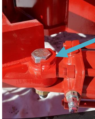
Anti-turn Base end of cylinder shown
